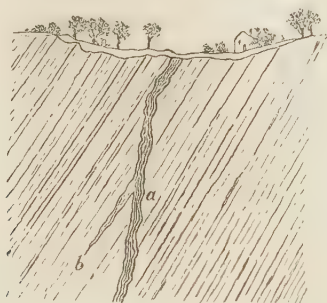
FIG. 15.—True vein a , sending out a branch b , corresponding with bedding.
